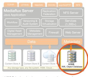
XODB is the database engine at the core of Mediaflux's services-oriented data mangement architecture.
